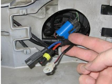
Route the cables from the ballast and ignitor through to the headlamp assembly.
