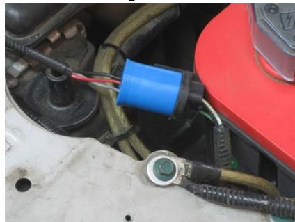
*Plug the harness into the OEM headlight connector (yours may differ slightly).*
