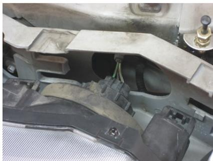
*Gently pull the headlamp assembly forward and unplug the headlight, being careful not to damage the retainers on the plug.*
