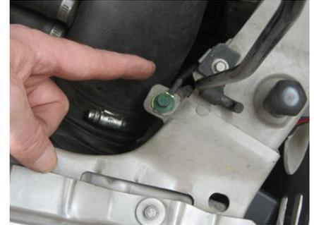
Ground the harness\* to the chassis or body on the passenger side
