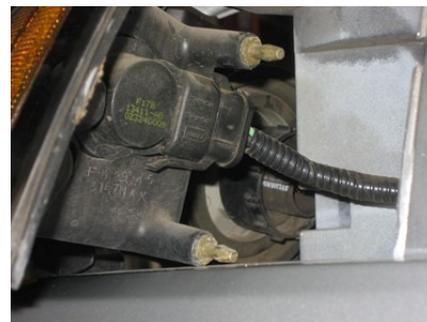
*Locate the parking lamp connector on the rear of the headlamp assembly and unplug it, also being careful not to damage the retainers on the plug.*
