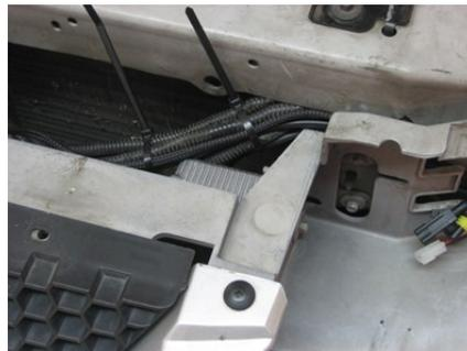
*Use cable ties to secure the wiring harness along its route.*
