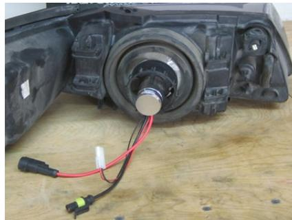
Install the Xenon bulbs, being sure not to touch or come in contact with the glass! Use the provided plastic covers to protect the stock bulbs with.
