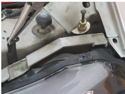
*Remove the retaining clips.*
