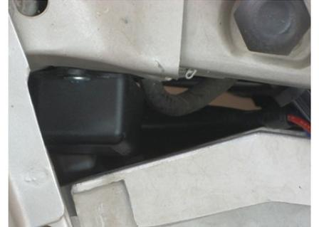
*Shown here is an ideal location for the ignitor, just behind the headlamp assembly mounting area.*
