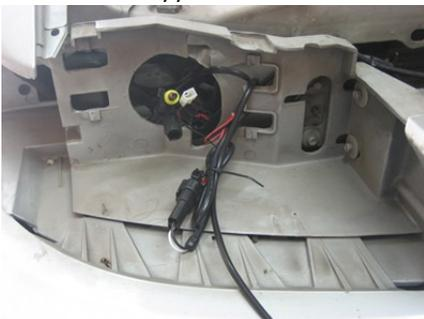
*Plug the harness into the passenger side ballast & bundle the excess if there is any.*
