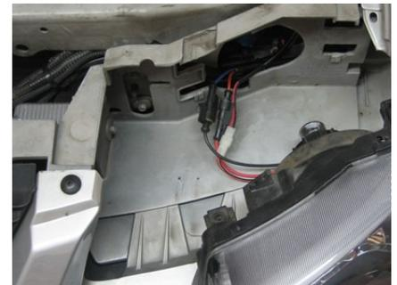
Plug the headlamp assemblies into the harnesses from the ballast and ignitor and reinstall them, being sure to plug the parking lamp harnesses back in!
