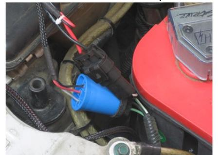
*Plug the harness into the driver's side ballast, then tuck these out of the way.*
