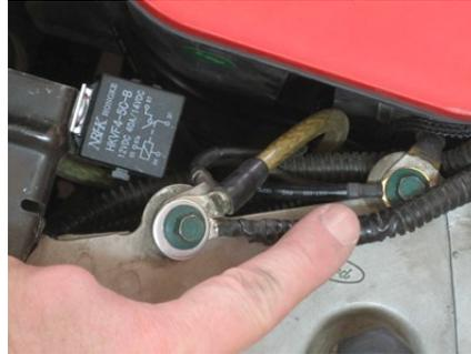
Ground the harness\* to the chassis or body on the driver's side.
