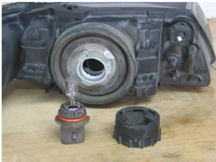
Carefully remove the stock bulbs by twisting the retainer counterclockwise. Once the retainer has been removed, pull the bulb straight out of the socket. \*\*
