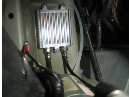
Shown is the ballast on the passenger side mounted to the underneath of the chassis with the provided screws.
