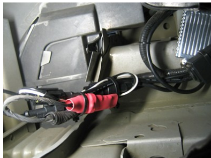
Shown is the completed installation on the drivers' side. Note that the ignitor is secured to the factory wiring harness.
