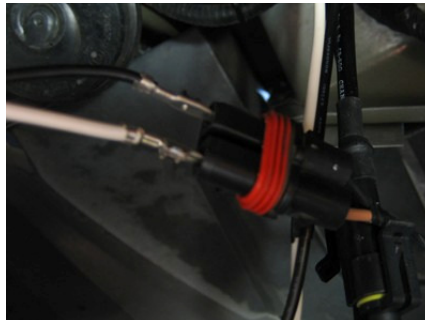
Plug the pin with the black wire into the ground pin on the factory plug. Plug the pin with the white wire into the power pin on the factory plug.**
