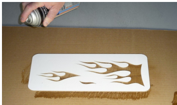
Step 1: Spray a release agent to ensure filler won't stick to template.
