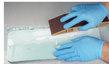
Step 3: Sand surface of filler to expose detail in template.
