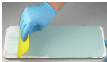
Step 2: Apply body filler to inside openings - build filler over entire template.
